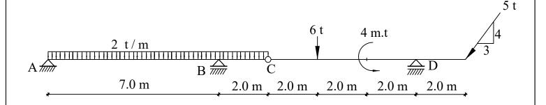
Q2) Draw the N.F, S.F, and B. M. Diagrams for the shown frame
